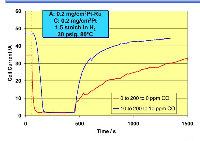
**Conclusion:** Alloy catalyst which exhibits reasonable tolerance to 10 ppm CO (without air bleed) experiences extremely long recovery time back to 10 ppm when exposed to 200 ppm CO
