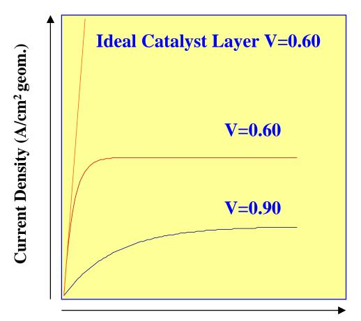
Loss in utilization with increasing thickness occurs because of increased ionic IR loss within the catalyst layer and/or limited oxygen permeation rate.
