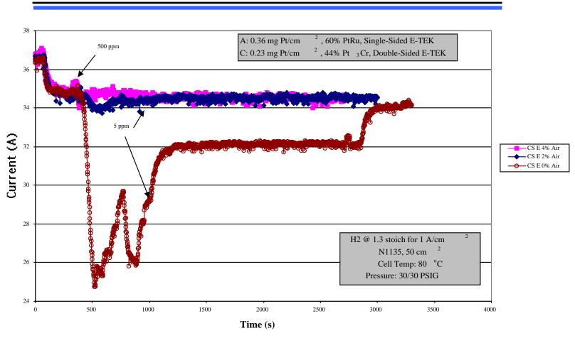
CO stepped from 500 ppm to 50 ppm @ 75 ppm/min; then from 50 ppm to 5 ppm @ 15 ppm/min
