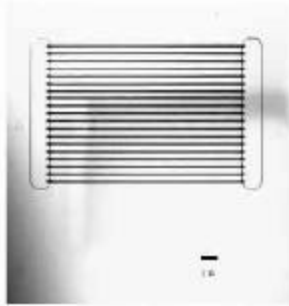
Figure 1 Simple Microchannel Array Consisting of Two Header Areas and Nineteen Flow Paths (Microchannels)
