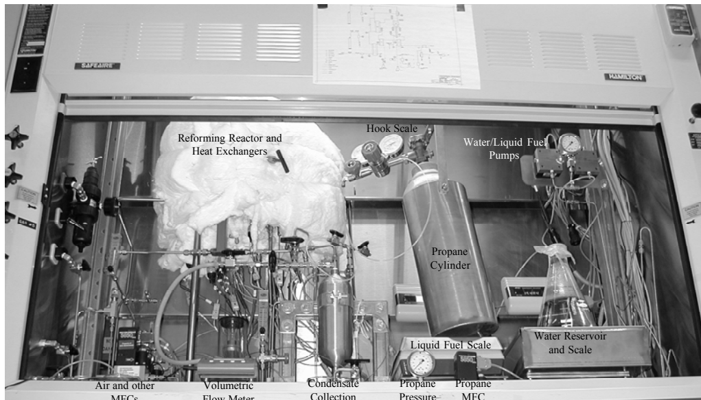
Figure 1. Experimental Test Stand Configured for Propane. The propane is suspended from a hook scale to monitor weight loss. Liquid fuels are placed in a reservoir on the platform scale.
