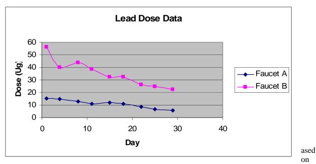
Section 9 of Standard 61, the higher the variability in the results, the more difficult it is to pass the test. Also, if the volume of water that a product contains is high (such as a faucet with a long neck) the resulting Q value will be high. Thus, a different choice of materials or technologies may be used for high-volume products.
