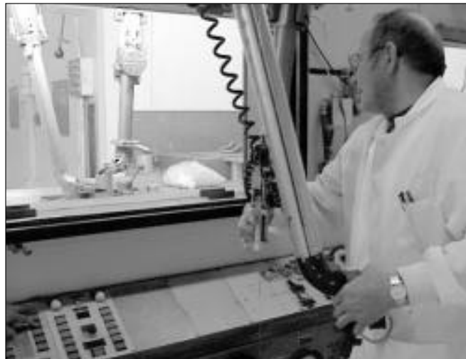
Marty Ott of Nuclear and Radiochemistry (CST-11) uses a pair of manipulators to handle an object in a dispensary cell at the Technical Area 48 Hot Cell facility. Facility managers are concerned that a disruption of electrical power will irreversibly damage the windows because the oil in the windows will coagulate; the interior of the facility must be maintained at a constant temperature above 40 degrees F to avoid this problem. Photo by John Bass
