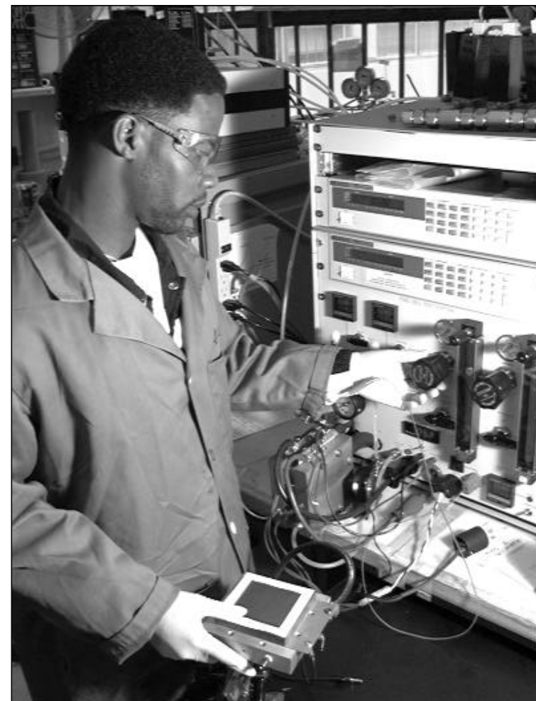
Tommy Rockward, a graduate research assistant in Electronic and Electrochemical Materials and Devices (MST-11), runs a test at a fuel cell testing station. He is collecting data to help determine the effects of impurities in the fuel stream on fuel-cell performance. Photo by LeRoy N. Sanchez
