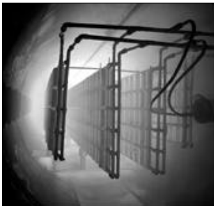
Inside the PSII process chamber aluminum automotive pistons are treated to improve their wear properties. The glow is from the argon gas ionized inside the chamber by radio-frequency fields.
