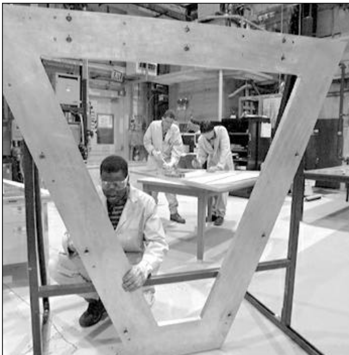
Craig Martin, foreground, kneels to smooth a portion of a detector frame, preparing it for its central mylar sheet and layers of electronic circuits. Behind him, at the table, are Javier Martinez (left) and Jay Pederson (right). Photo by LeRoy Sanchez
