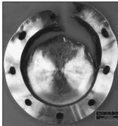
At top, The results of a hemispheric impact on high explosives show that at 65.5 meters per second the high explosive, in this case PBX 9501, is deformed, but no energetic reaction is observed. At bottom, impacted at 80.7 meters per second, however, a separate sample reacts violently, breaking the sample holder. Photos courtesy of DX
