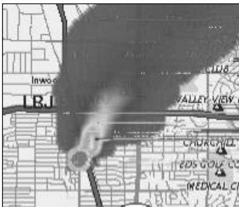
This simulation of a toxic release in the Dallas area shows the expansion of a ground-level plume. The work is being conducted under the Lab's Urban Security Initiative.
