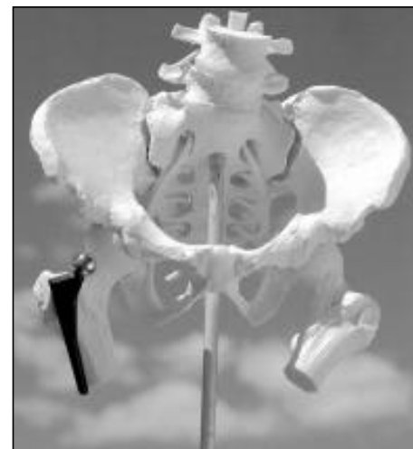
A prosthetic carbon hip, shown half-size on the right side of a full-size human pelvic structure, may one day replace currently used metal joints.
