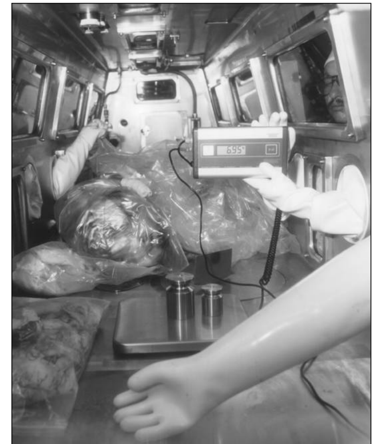
Ricky Baros of CST-7 uses weights to calibrate a scale in a glove box. Wastes such as those shown in the plastic bags are separated by type and then weighed before packaging in drums. The bag in the lower left corner of the photo contains rags.
