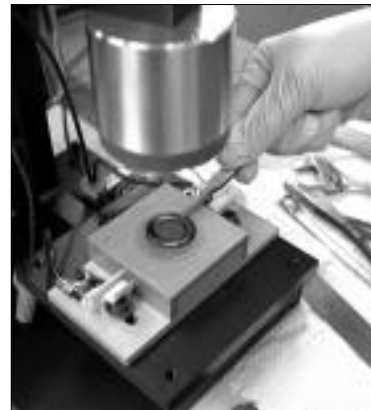
Encapsulating the ultracapacitor core. Photos by LeRoy N. Sanchez
