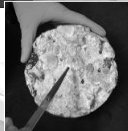
Bill Carey, left, rinses chemicals off a concrete core held by George Guthrie, before examining the core for the presence of alkali-silica reaction. Inset: An eyedropper is used to apply stain to a concrete core. The darker areas of the concrete core show where alkali-silica reaction has occurred. Photos by James E. Rickman
