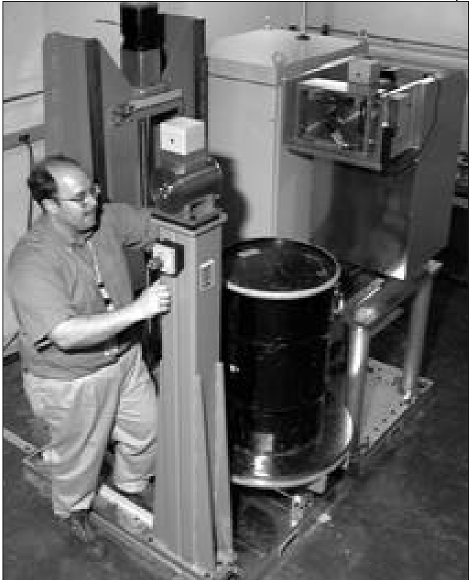
Tom Prettyman of Safeguards Science and Technology (NIS-5), chief scientist and project leader for the Lab's Tomographic Gamma Scanner project in support of clean-up efforts at Rocky Flats, makes an equipment adjustment on a skid-mounted TGS. The 30-gallon drum in the center of the device shows where a sample would be placed to be assayed by the equipment. Photo by LeRoy N. Sanchez
