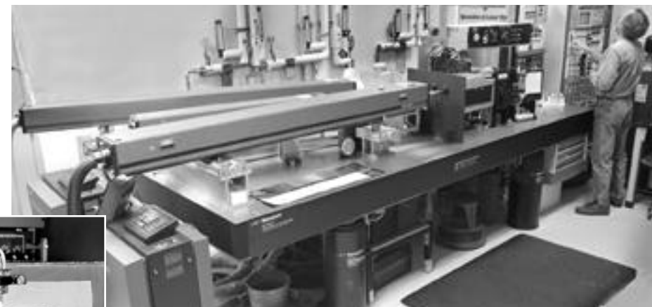
Above: Robb Habbersett checks the readings on the 13-foot-long array of lasers, chambers, tubing, electrodes, sensors and other sophisticated electronics that make up a flow cytometer known locally as "Big Geek." The device, which is operated by Habbersett, analyzes, sorts and characterizes cells, chromosomes and other biological samples. Photos by Fred Rick
