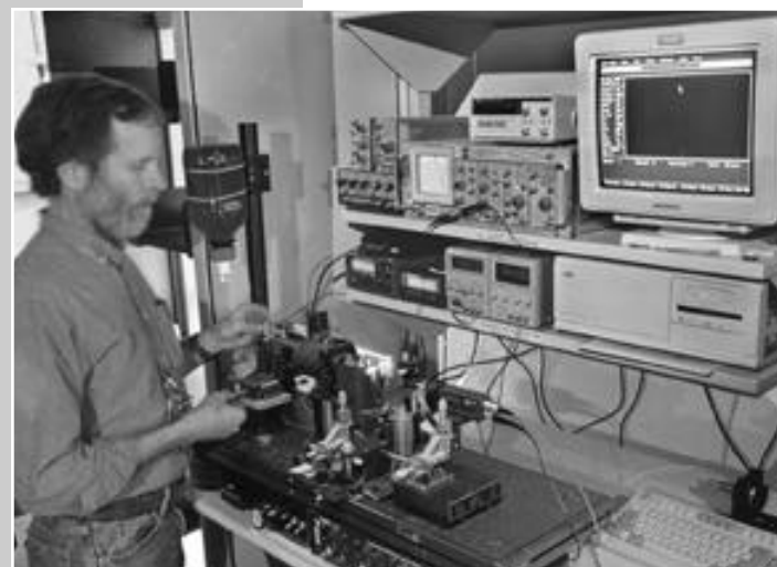
Robb Habbersett of Cytometry (LS-5) sets the instruments on "Little Geek," a new 3-foot-long flow cytometer that can be used to analyze single molecules, one of many technological advances the Laboratory has made in the field of flow cytometry since the 1960s.
