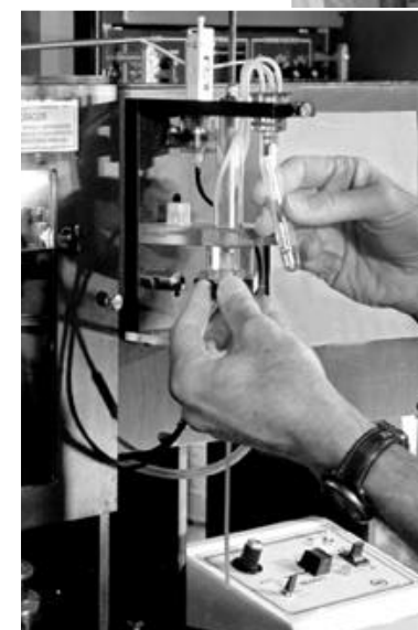
Above: Robb Habbersett checks the readings on the 13-foot-long array of lasers, chambers, tubing, electrodes, sensors and other sophisticated electronics that make up a flow cytometer known locally as "Big Geek." The device, which is operated by Habbersett, analyzes, sorts and characterizes cells, chromosomes and other biological samples. Photos by Fred Rick
