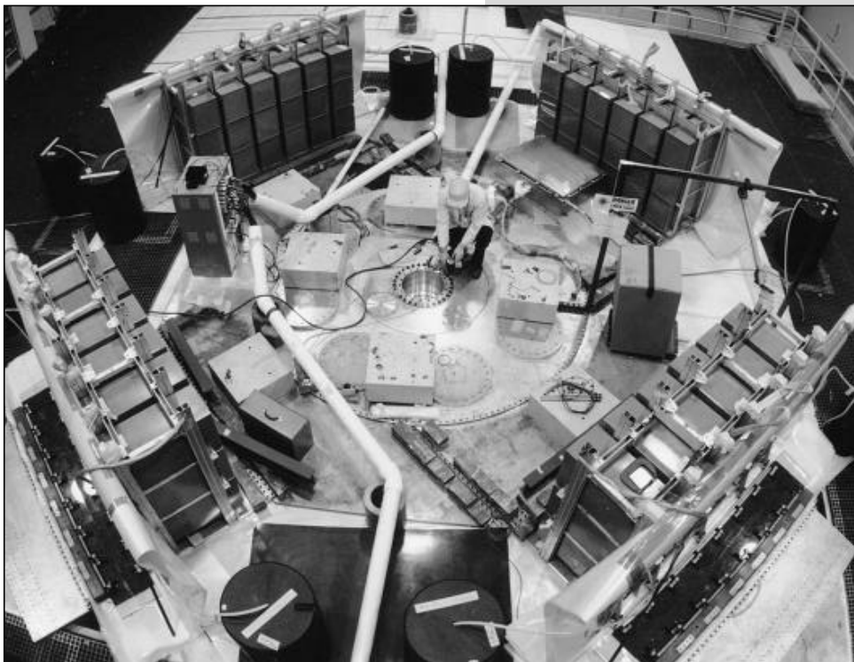
Ringed by capacitor banks that could achieve 4.3 megajoules of stored energy, Pegasus II, shown in this file photo, was once one of the largest capacitor-bank facilities in the world.
