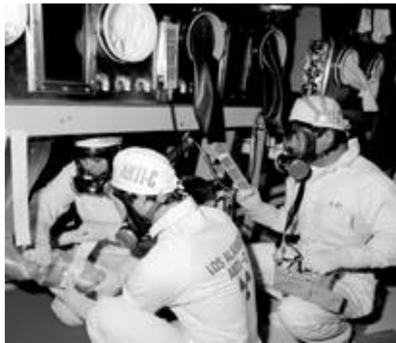
Two employees of TA-55's Plutonium Facility (left and center) remove material from a glovebox in what's called a bagout procedure while a radiation control technician monitors the procedure for contamination. File photo
