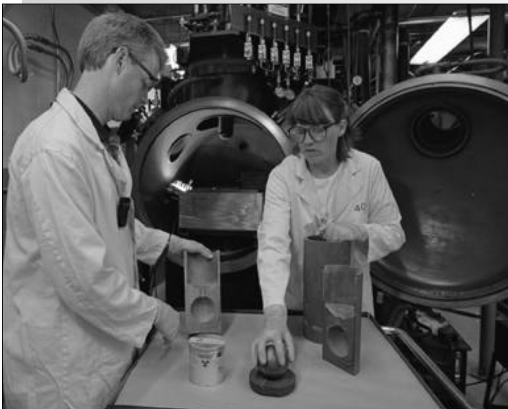
Researchers Doug Kothe, left, and Deniece Korzekwa of the Materials Science and Technology (MST) Division stand in front of a plasma furnace with a cast sphere of depleted uranium and its mold. Kothe is helping develop a computer tool that models and simulates the casting process of alloys used in weapons parts. The Telluride simulation tool also will benefit private industries that cast complex metal parts, such as engine blocks. Photo by LeRoy N. Sanchez
