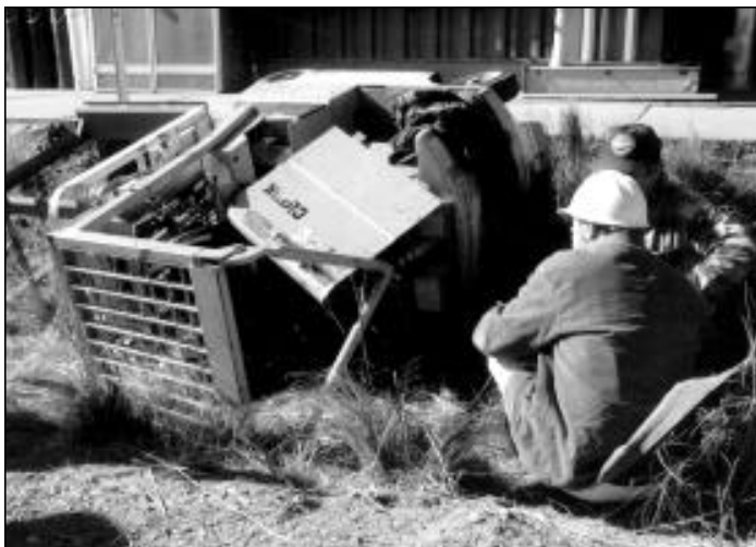
Inspectors examine a forklift that went off a walkway at Technical Area 35, resulting in serious injury to the Engineering Sciences and Applications (ESA) Division employee who was driving it. Photo courtesy of ESA Division.
