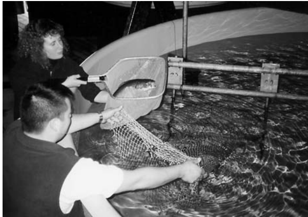
Figure 2a. Fisheries Behavioral Ecology staff inserting sablefish into a net to be towed to simulate capture in a trawl codend.
