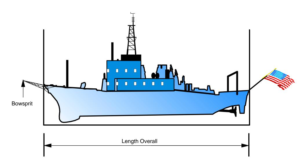
Figure 6 to Part 679. Length Overall of Vessel (see § 679.2)
