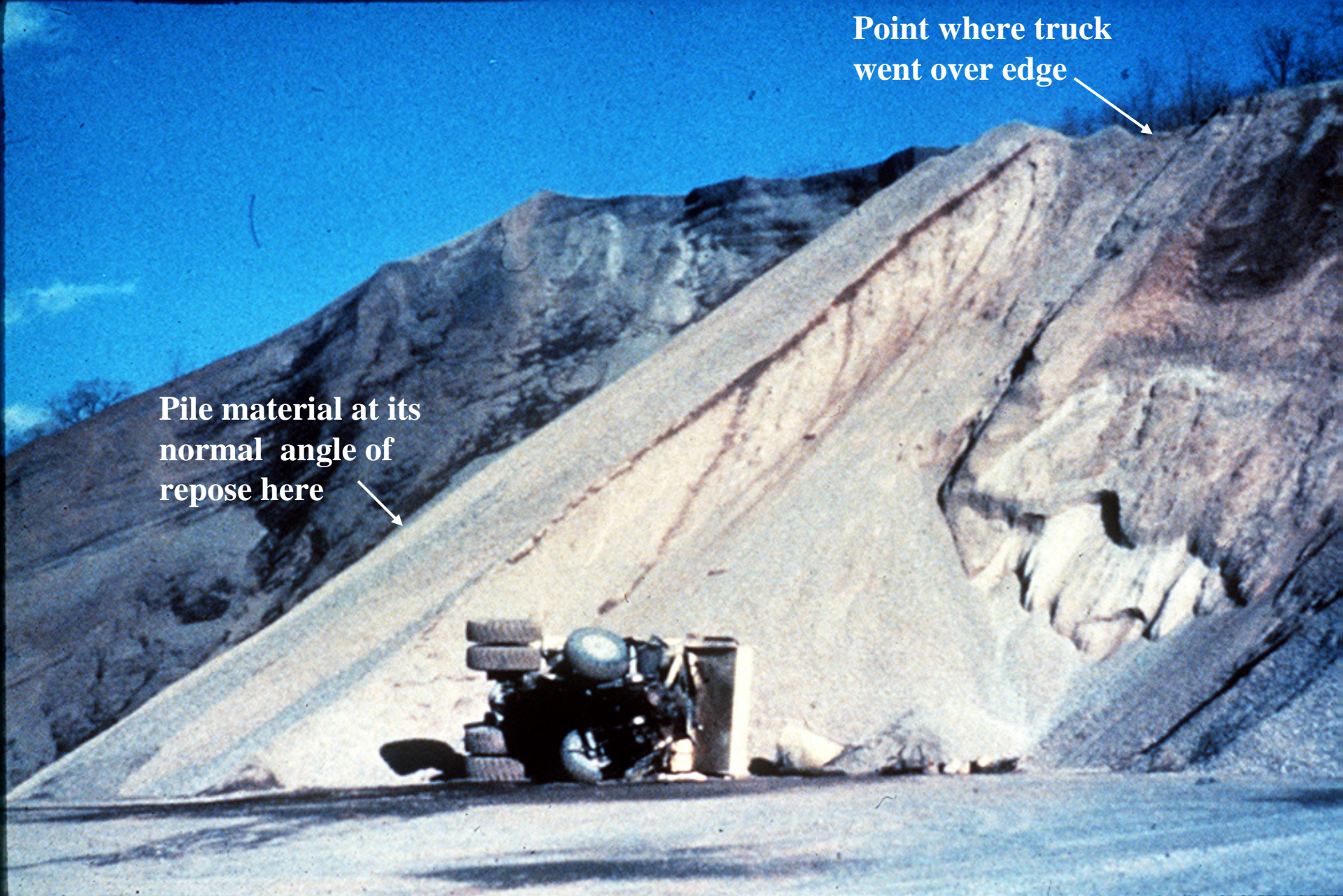
In this accident the pile was 70 feet high pile. Where the truck went over the edge, the pile had been loaded out and made steeper than the material's normal angle of repose. This is a common feature in many dump-point accidents.
