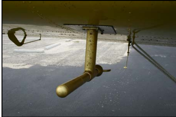
Figure 2: Front view of AIMMS-20 mounted on the AT402 HI-RISE aircraft.
