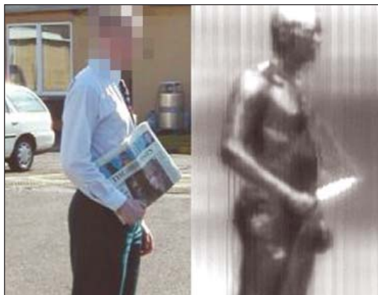
Spot the knife? Millimeter waves, close to terahertz, show their ability to see through clothes and paper.
