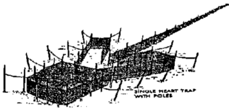
FIGURE 14. POUND NET (West et al. 1994)
