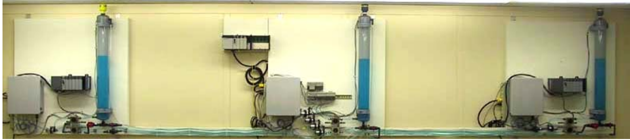
Figure 4 - Water Distribution SCADA System
