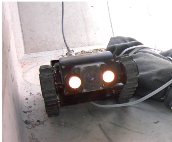
Figure 5a. Shape-shifting robot in lower configuration.
