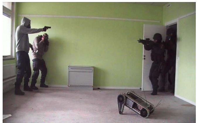
Figure 3. Tactical test of the distraction-siren. From left to right: the officer acting as criminal; the officer acting as hostage; the two SWAT-officers attacking. The hostage taker was instructed to shoot at the police, which he succeeded in despite the siren. The hostage immediately plugged his ears with his fingers. The electronically filtered hearing protection used by the police protected them from the noise.
