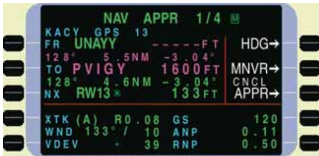
Figure 1-15. FMS Control Display Unit. This depicts an aircraft established on the Atlantic City, NJ, RNAV (GPS) Rwy 13 instrument approach procedure at the Atlantic City International Airport, KACY. The aircraft is positioned at the intermediate fix UNAYY inbound on the 128 degree magnetic course, 5.5 nautical miles from PVIGY, the final approach fix.
