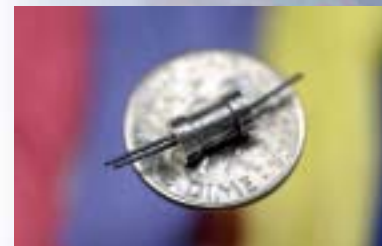
Our integrated fuel reformer, the smallest in the world, is an example of the type of miniaturization of integrated chemical and thermal processes that is possible through exploitation of microscale phenomena.
