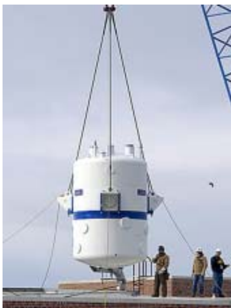
This superconducting magnet is a part of the 900-MHz wide-bore nuclear magnetic resonance (NMR) spectrometer at EMSL. This spectrometer is now operational and is one of the world's most powerful and sensitive instruments for chemical, biological, and materials research.
