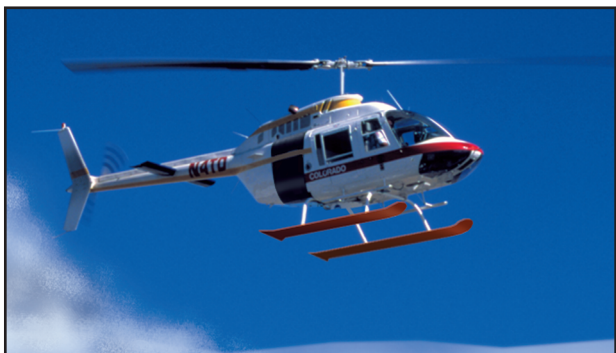
Figure 9-6. Ski equipped helicopter.
