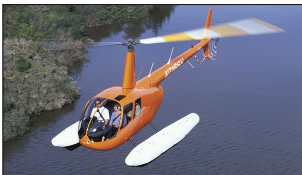
Figure 9-1. Float equipped helicopter.
