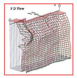
Using a profiler in combination with a bore hole probe, (see <u>Balance your Explosives - Borehole Probes</u>), a blaster can actually measure the volume of material that each explosive charge is expected to affect. This way, charges can be adjusted accordingly from hole to hole, or even within portions of the same hole.
