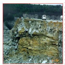
The initial calculation in determining the volume of material being blasted typically involves determining the "burden." Burden is the distance between the bore hole and the area-of-relief. Often, burden is visually estimated because of the inherent difficulty in measuring the face. In other cases, a "burden pole" is used in conjunction with a measuring tape to determine the "maximum burden" in a certain area of
