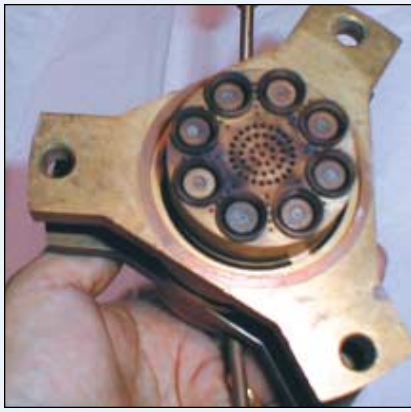
Macrolaminated fuel injector array, shown here after testing, is used for dual-fuel applications – Photo courtesy of Parker Hannifin
