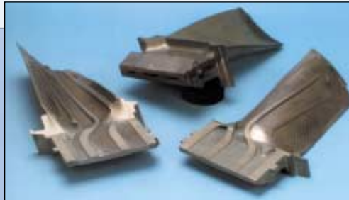
Fabricated blade, showing complexity of internals
