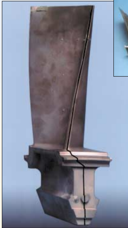
Fabricated blade showing bonding plane
