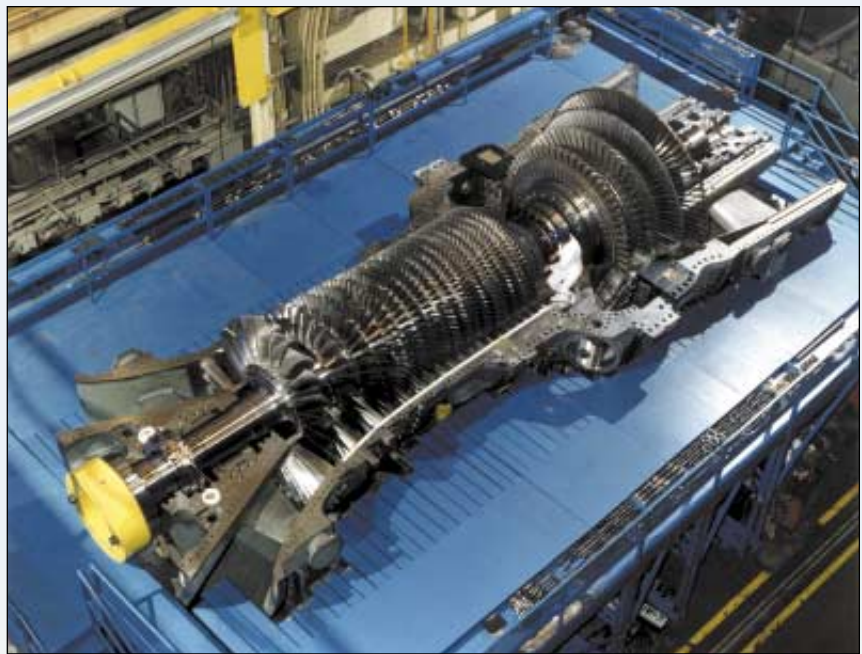
General Electric's H System™ gas turbine showing the 18-stage compressor and 4-stage turbine
