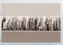
Thermoelectric materials like these silicon nanowires are capable of transforming waste heat into electricity. While promising, these materials require greater stability at elevated temperatures and greater efficiency for use in fossil energy conversion systems.
