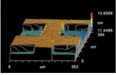
Studying patterned electrodes such as this one, prepared using a combination of lithographic techniques and magnetron sputtering, have led to significant improvements in oxygen-reduction electrodes. The ability to reduce oxygen at the interface of the cathode and the electrolyte addresses a key factor that limits performance of fuel cells, oxygen separators and certain sensors.
