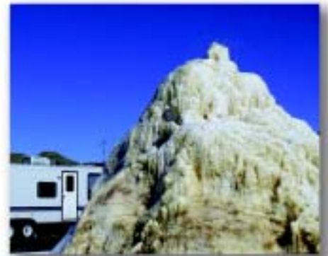
During the FTE ® separation process, ice piles separate into produced water and brine.
