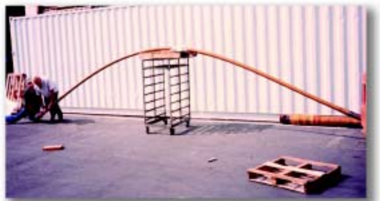
Engineers demonstrate the flexibility of the advanced composite drill pipe.
