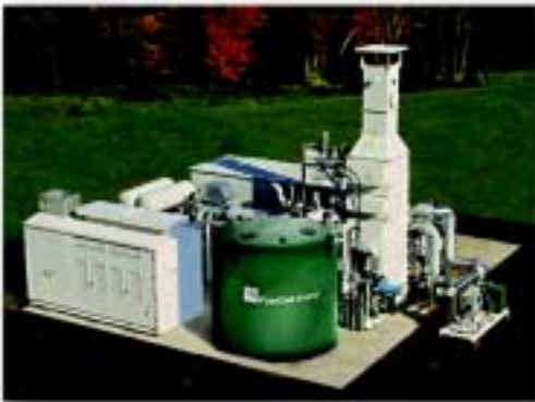
Testing of a 1-MW FuelCell Energy MCFC Plant
