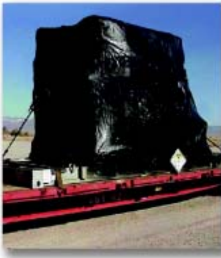
Furnace Packaged With Spray-On Polyurea Coating for Shipment to the Nevada Test Site
