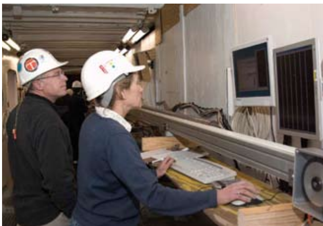
Physical property specialists Philip Long (PNNL) and Anne Tréhu (Oregon State University) operate an infrared camera on the catwalk of the JOIDES Resolution. The infrared camera helps the scientists identify which portions of the core contain gas hydrate.
