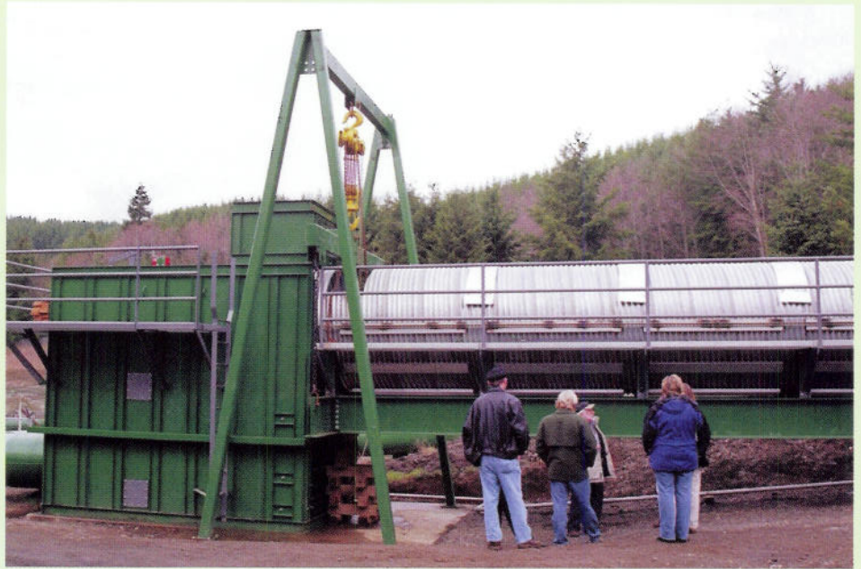
The culvert test bed allows researchers to evaluate current culverts and future retrofits.
