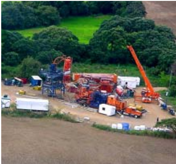
Example of a coiled tubing drilling rig currently used by Schlumberger. In this project a “built-for-purpose” microhole coiled tubing drilling rig will be developed and built that has a small footprint, is easy to move, and fast to mobilize.
