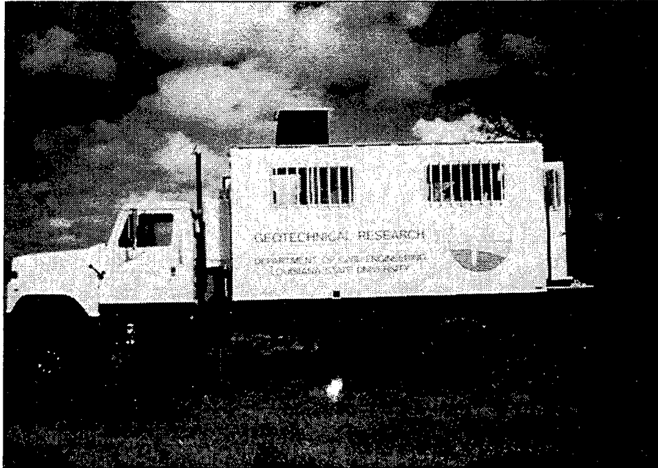
Figure 5-7: Self-Contained CPT Truck (Photo courtesy of M. Tumay of Louisiana Transportation Research Center)
