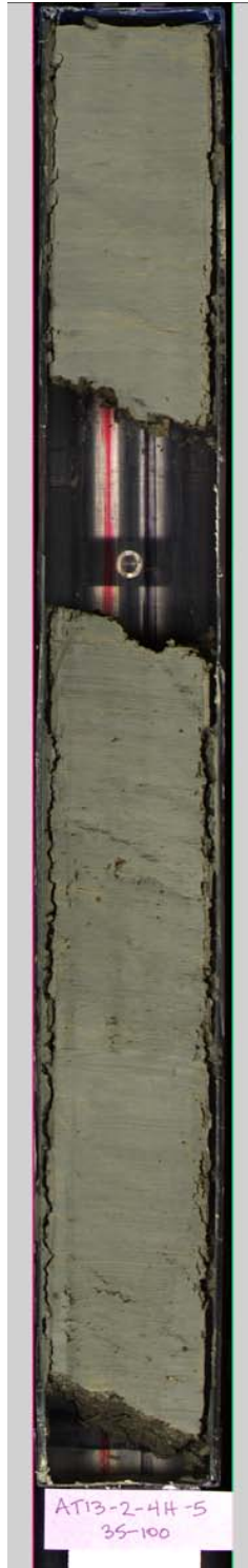
Figure AT-8. Line scan color image taken with the MSCL-XYZ using the Geoscan camera of a typical core section seen during the GOM-JIP Expedition (Section AT13-2-4H-5): clay with gas expansion voids. Pixels are 100 microns on a side. Color fringing on edges of image results from registration of camera CCDs.
