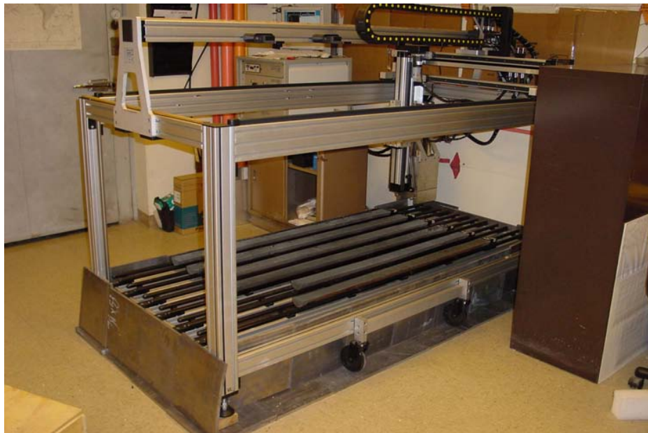
Figure EXPL-16. MSCL-XYZ installed in the DSDP West Coast Repository at the Scripps Institution of Oceanography, where the split cores from the GOM-JIP were logged. The MSCL-XYZ is configured for natural gamma measurements in this photo.
