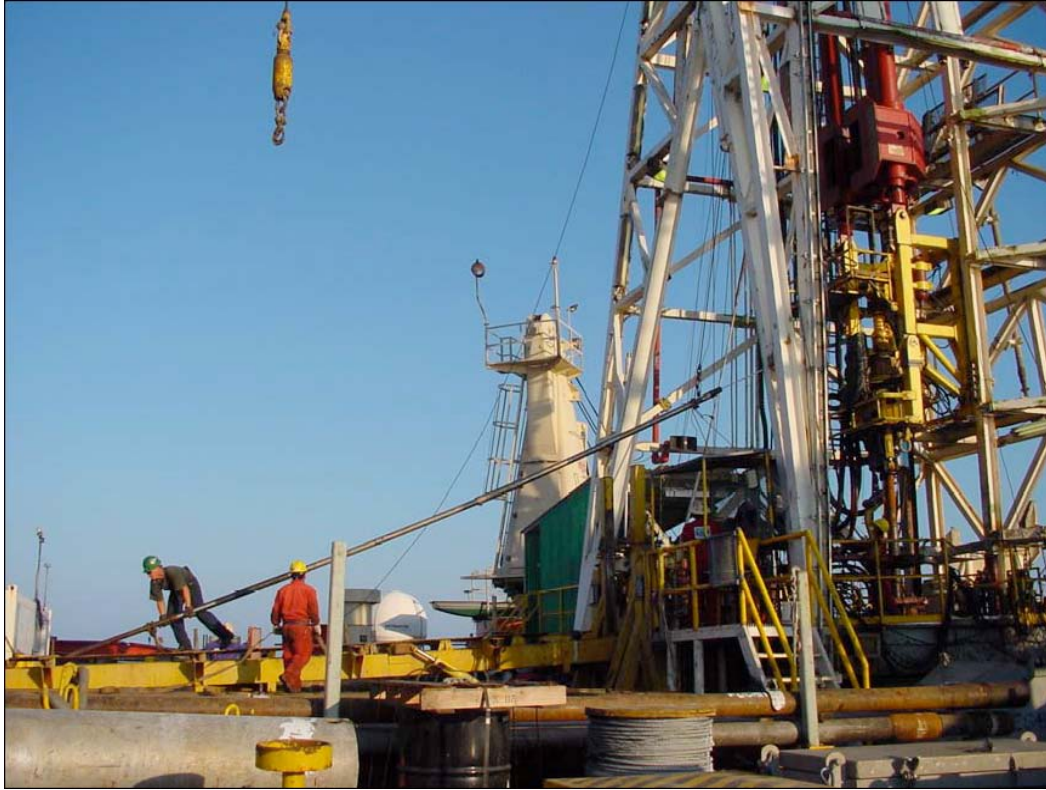
Figure EXPL-1. Fugro Pressure Corer (FPC) being deployed on the Uncle John during the GOM-JIP Expedition.
