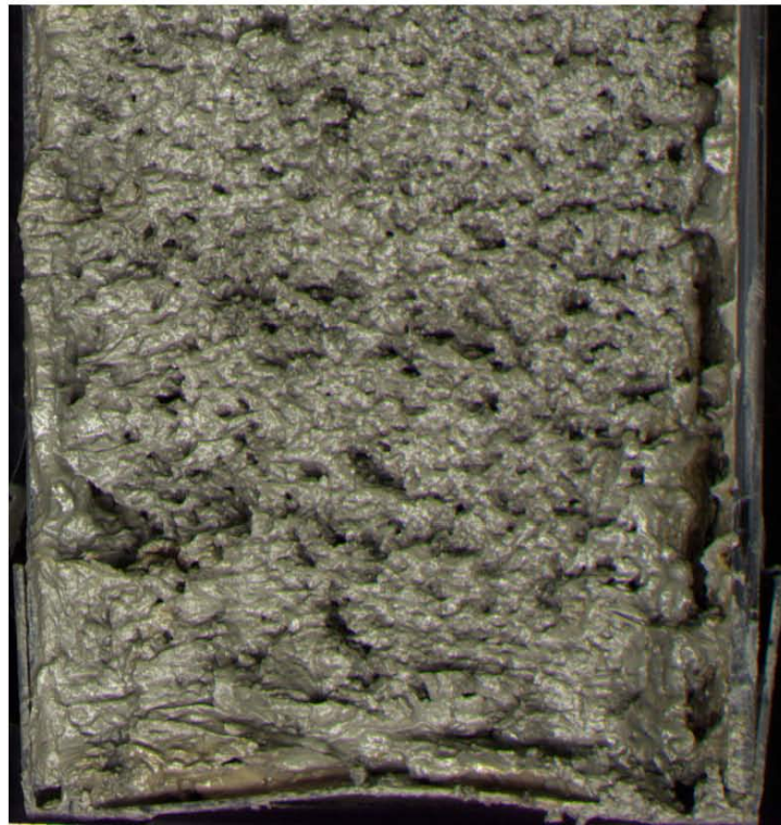
Figure INT-1. Moussy core, showing frothy, wet texture indicative of hydrate dissociation. Core at top, containing massive hydrate as well, is from ODP Leg 204. Core at bottom is from the GOM-JIP, ATM1-5H-2, 70-75cm.
