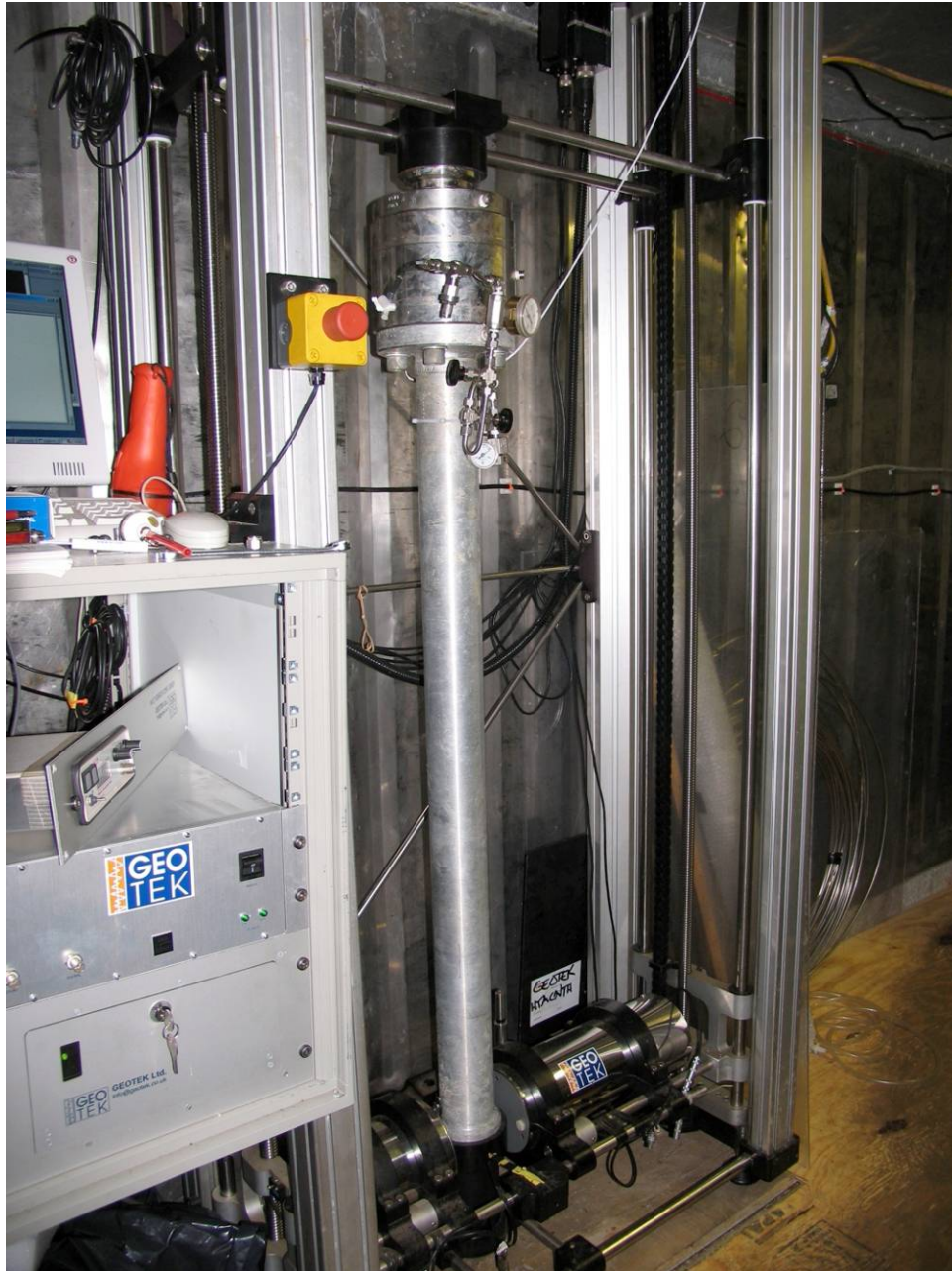
Figure EXPL-4. HYACINTH Storage Chamber in place and ready to be logged in the MSCL-V, inside the 20-foot refrigerated logging container on the Uncle John during the GOM-JIP Expedition.
