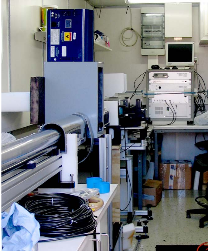
Figure EXPL-13. MSCL-S inside the 20-foot unrefrigerated logging container on the Uncle John during the GOM-JIP Expedition.
