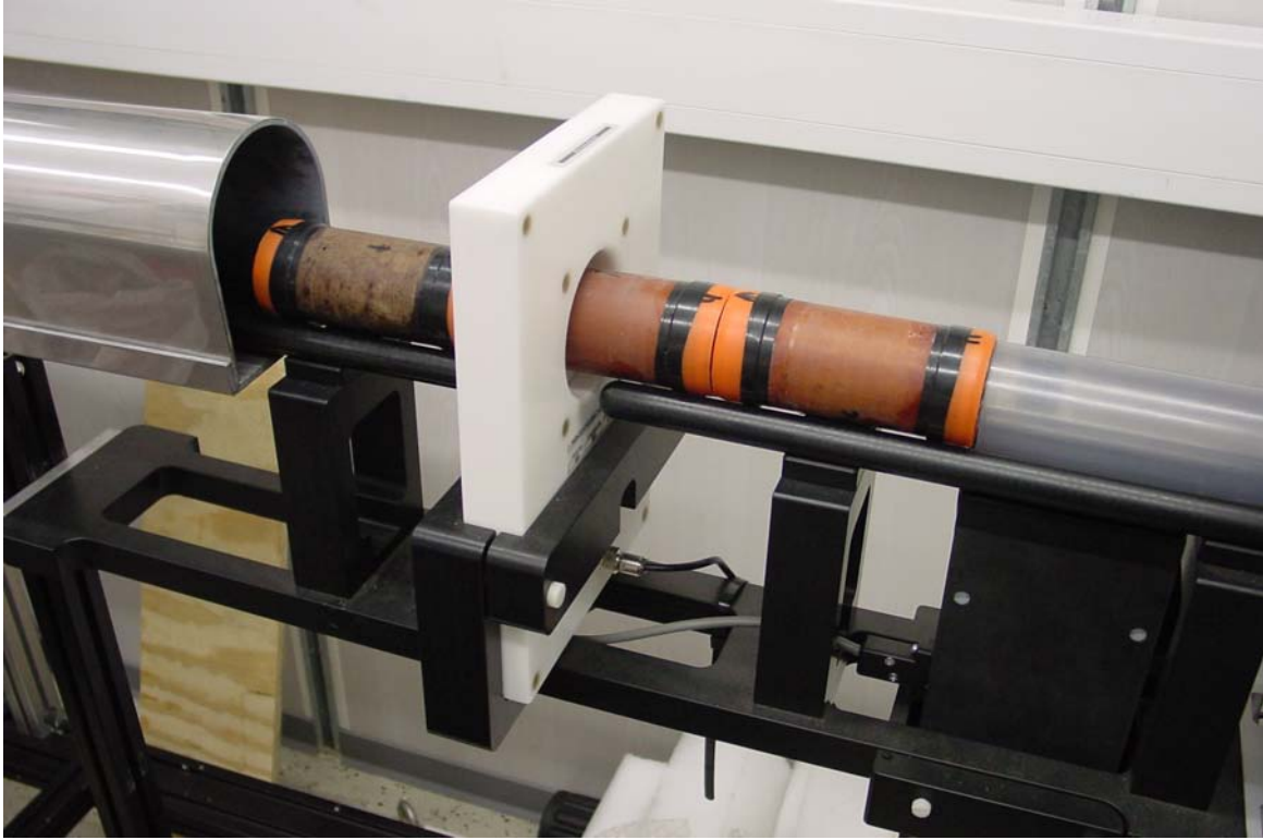
Figure AT-10. ROV push core AT14-7PC, collected in fiberglass liner, in the MSCL-S. Small fiberglass core sections had end-caps taped on for logging to prevent the core from oozing out of the liner.
