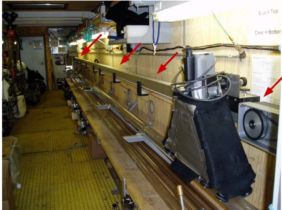
Figure EXPL-5. The infrared imaging track (red arrows) set up along the length of the 40-foot core processing container, above the core rack. The track was driven and the data acquired and displayed by the Geotek Infrared Imaging software.
