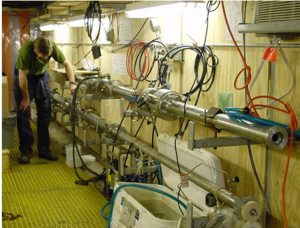
Figure EXPL-3. HYACINTH Storage Chamber, connected to the Shear Transfer Chamber & Manipulator (top) and MSCL-P (bottom) in the 40-foot refrigerated core processing container on the Uncle John during the GOM-JIP Expedition.
