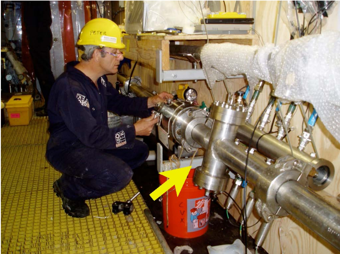
Figure EXPL-15. MSCL-P with Geotek P-wave Central Measurement Chamber in place (yellow arrow). The Georgia Tech measurement chamber (not in use) is sitting behind the Geotek CMC.
