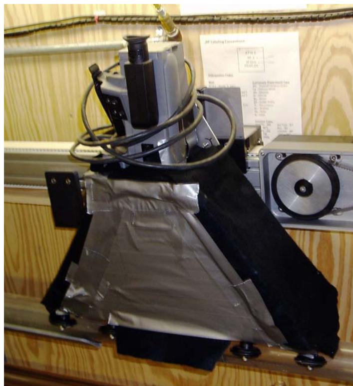
Figure EXPL-6. The FLIR ThermoCam SC2000 camera, mounted on its wheeled skate and covered with black felt to cut out reflected infrared radiation.
