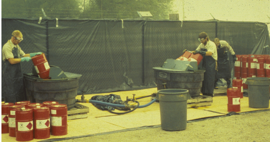
Figure 6-1. Lampricide (TFM, 3-trifluoromethyl-4-nitrophenol) application apparatus showing treatment personnel loading Lampricide® into mixing tanks during the 1994 treatment of the Manistee River in northwestern lower Michigan.
