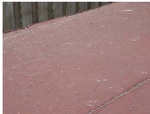
Figure 4d. Explosion/fire-associated debris (grit-like material) on hot tub cover, Romulus, Michigan (8/12/05). (EPA contractor photo.)
