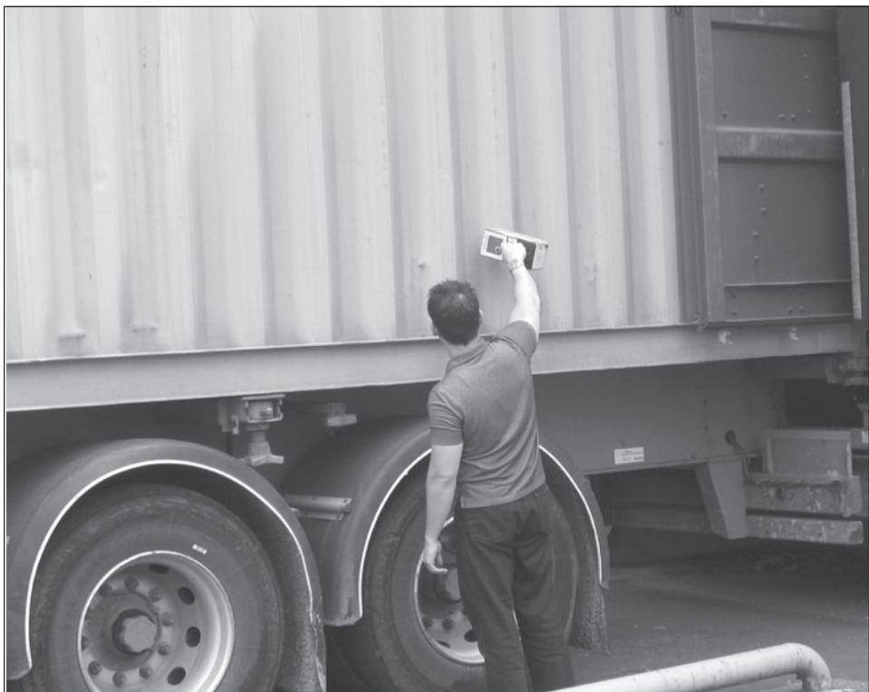
Figure 9: CBP Official Using Radiation Isotope Identifier Device to Examine Container at CSI Seaport
