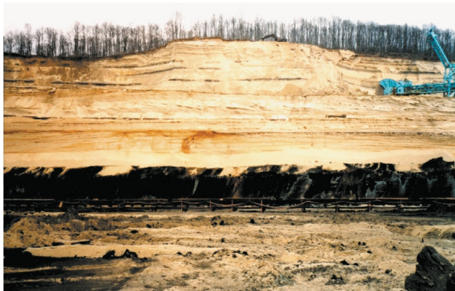
Figure 2. Opencast coal (Pliocene lignite) mine located in the main Romanian BEN-affected area. Most visible is coal layer #1V (dark brown, ~25 feet thick), which underlies the entire affected area.
