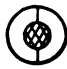
FIG. 9. The form of the maximal semisimple diagrams ( n > 2 ); the hatched circle is to be filled with all (n - 2) -loop chains.
