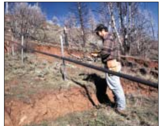
Above: Testing a solar-powered radio telemetry system for remote transmission of real-time landslide data (Photo: Mark Reid, USGS)
