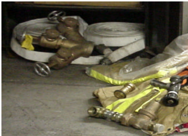
Example of manifolds, fire hoses and nozzles commonly used.
