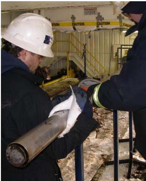
Figure 9: Cutting inner core barrel into 3 foot core segments in pipeshed. Core end is visible lower left side of photo.
