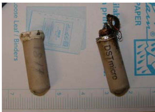
Figure 20: DSTmicro capsule data logger used to record time, temperature, and pressure during coring and during MDT logging operations. Data logger on right was destroyed during operations outside capsule pressure rating.
