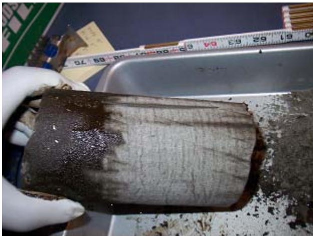
Figure 17: Whole core sample is scraped to remove oil-based drilling mud contamination.
