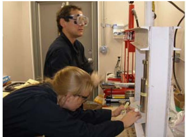
Figure 19: Core press to obtain interstitial water samples.
