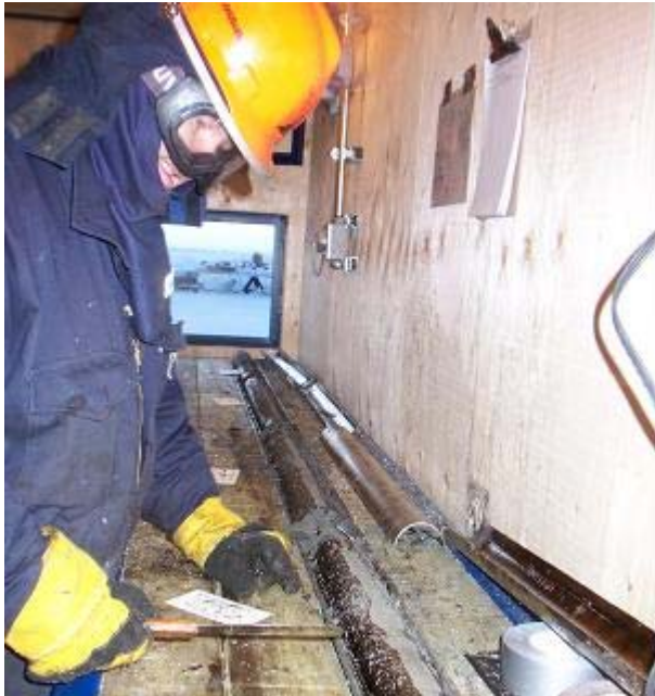
Figure 12: Core layout processing in “cold” trailer.
