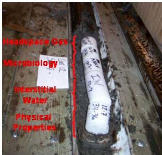
Figure 12: Core layout processing in “cold” trailer.
