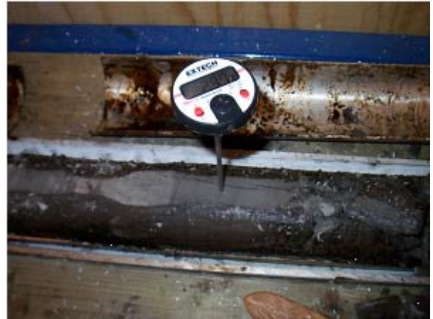
Figure 14: Temperature probe testing used to show decreasing temperature with time during gas hydrate dissociation in hydrate-bearing core samples during onsite subsampling.
