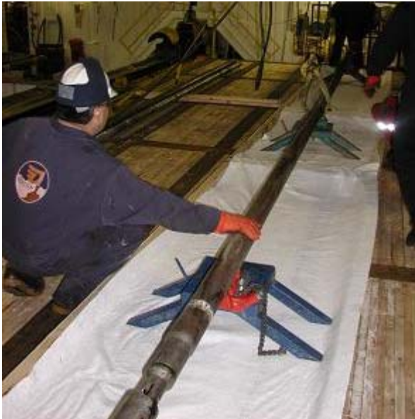
Figure 8: Core barrel inner liner separation in cold pipeshed processing area. Rig mats on pipe racks provided working surface.
