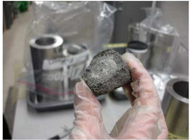
Figure 18: Cleaner innermost portion of core prior to placement into drill-press to remove formation water for later laboratory analyses.
