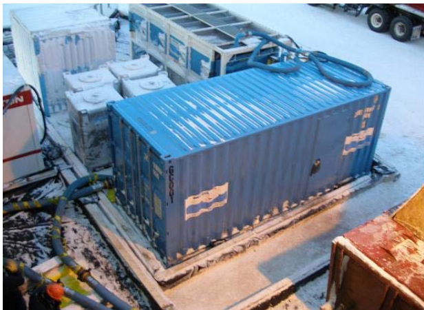
Figure 7: DrillCool, Inc. Heat Exchange Mud Chilling Unit onsite at Mount Elbert-01 Ice Pad.
