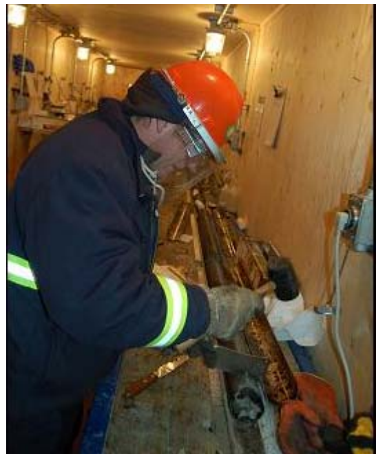
Figure 11: Subsampling gas hydrate-bearing core in core processing “cold” trailer.
