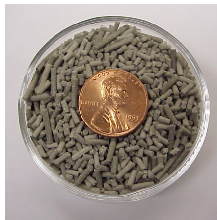
NETL CO 2 sorbent extrudates prepared at a commercial facility (Süd-Chemie Inc.)
