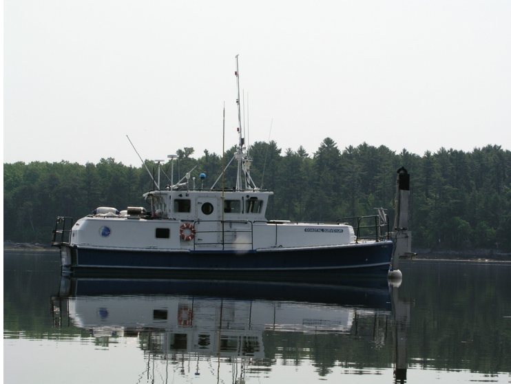
Figure 5 – University of New Hampshire R/V Coastal Surveyor. Note the adjustable bow ram which allows the hard mounting of a variety of sonar heads or other scientific equipment.
